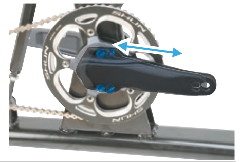
3 Crank adjustable (max 20mm)
